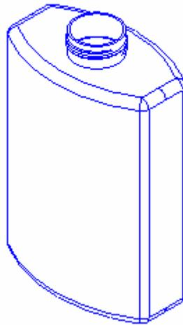
In the tutorial we will create, step-by-step, a function that will model a bottle as shown above. You will find the complete source code of this tutorial, including the very function `MakeBottle` in the distribution of Open CASCADE. The function body is provided in the file `Tutorial/src/MakeBottle.cxx`.
