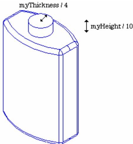
To position the cylinder, you need to define a coordinate system with the `gp_Ax2` class defining a right-handed coordinate system from a point and two directions - the normal and the X direction (the Y direction is computed from these two).
