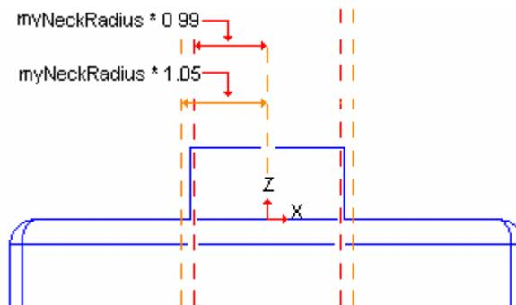
Notice that one of the cylindrical surfaces is smaller than the neck. There is a good reason for this: after the thread creation, you will fuse it with the neck. So, we must make sure that the two shapes remain in contact.
